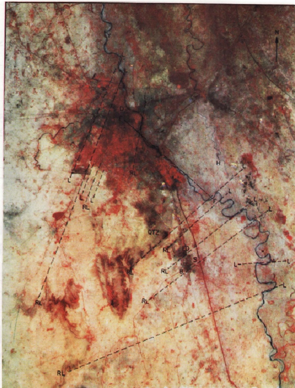
Fig. 3. (A) Lineaments and their relation with channel pattern of the Yamuna River (Y) in Delhi (D), Faridabad (Fd), Region. S- Sihi, B-Ballabhgarh, H-Hindan River, RL-Ridge Lineament, Ff-fault, Qtz-quartzite.
