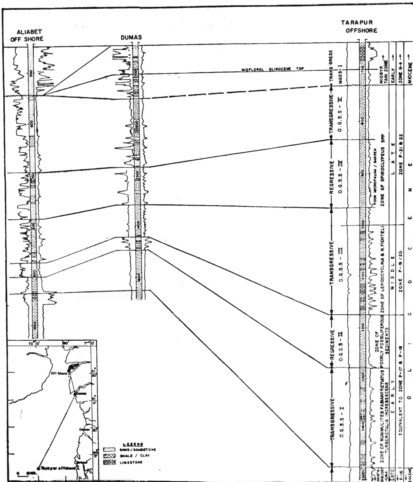
Fig. 1. Correlation of Oligocene strata: Gujarat subsurface & Tarapur offshore
